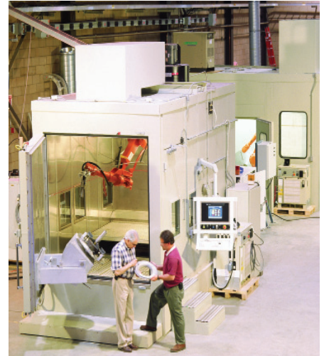
Among the advanced plasma control options available with Net Energy are the integrated PC/PLC-based Model 7700AP UPC (above) and the unique PlazJet II, a high power plasma spray process controller.
